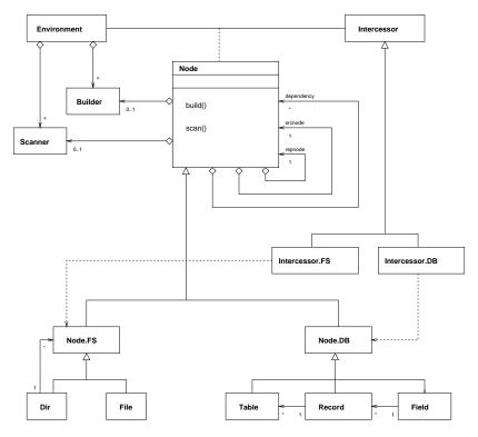
The point of SCons is to manage dependencies between arbitrary external objects. Consequently, the Build Engine does not restrict or specify the nature of the external objects it manages, but instead relies on subclass of the Node class to interact with the external system or systems (file systems, database management systems) that maintain the objects being examined or updated.
